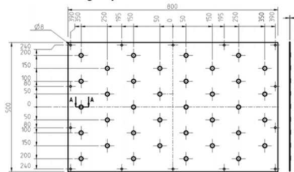
**Figure 1.** Dimensions of the inlet part of the air ducts, distances given in mm. The upper air duct has outlet suction along the two 800mm sides.
