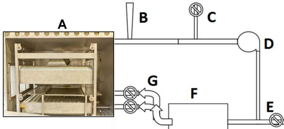
**Figure 2.** Schematic of the air heating system. A - the oven chamber, B - humidity sensor, C - air intake, D - ventilator, E - air out, F - heating unit, G - separation into top/bottom heat ducts.
