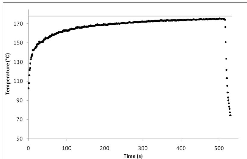
**Figure 4.** The black dots show the air temperature in the batch oven near the products, during the 8.5 min baking. The grey line indicates the initial oven temperature of 178°C.
